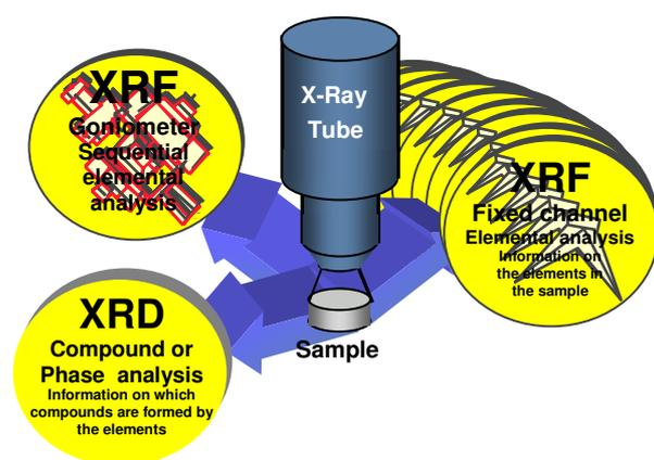
Figure 3: Integration of XRF and XRD in the same instrument: one sample, one instrument, one analysis
