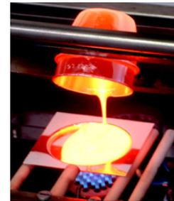
Figure 1: Fusion bead preparation
